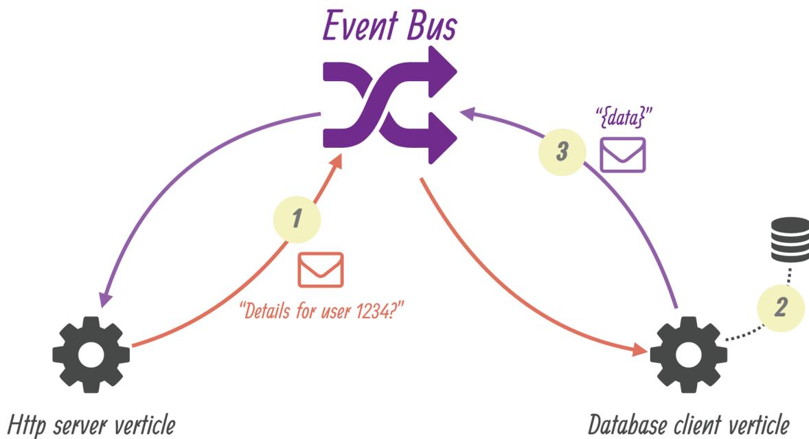
The event-bus allows passing any kind of data, although JSON is the preferred exchange format since it allows verticles written in different languages to communicate, and more generally JSON is a popular general-purpose semi-structured data marshaling text format.
