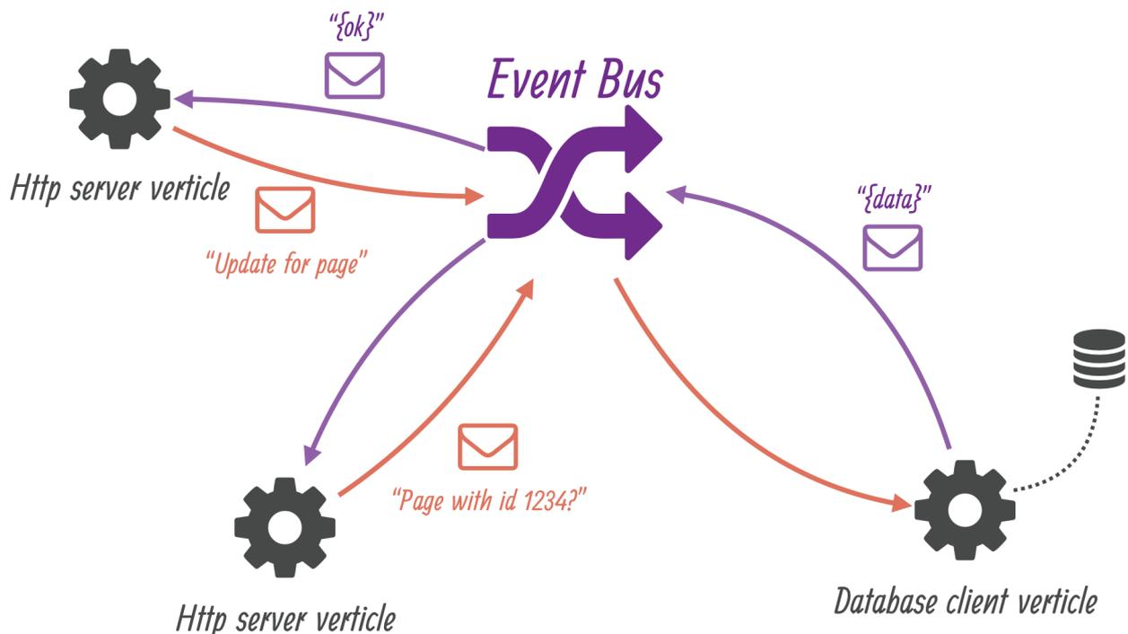
We will deploy 2 verticles to deal with HTTP requests, and 1 verticle for encapsulating persistence through the database. The resulting verticles will not have direct references to each other as they will only agree on destination names in the event bus as well as message formats. This provides a simple yet effective decoupling.
