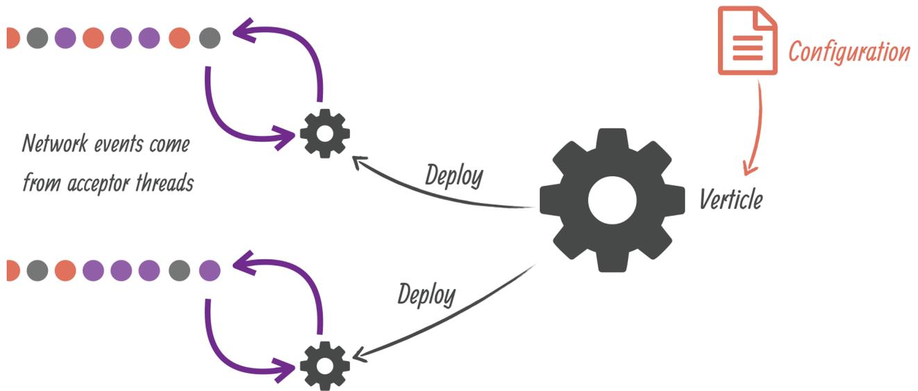
Incoming network data are being received from accepting threads then passed as events to the corresponding verticles. When a verticle opens a network server and is deployed more than once, then the events are being distributed to the verticle instances in a round-robin fashion which is very useful for maximizing CPU usage with lots of concurrent networked requests. Finally, verticles have a simple start / stop life-cycle, and verticles can deploy other verticles.
