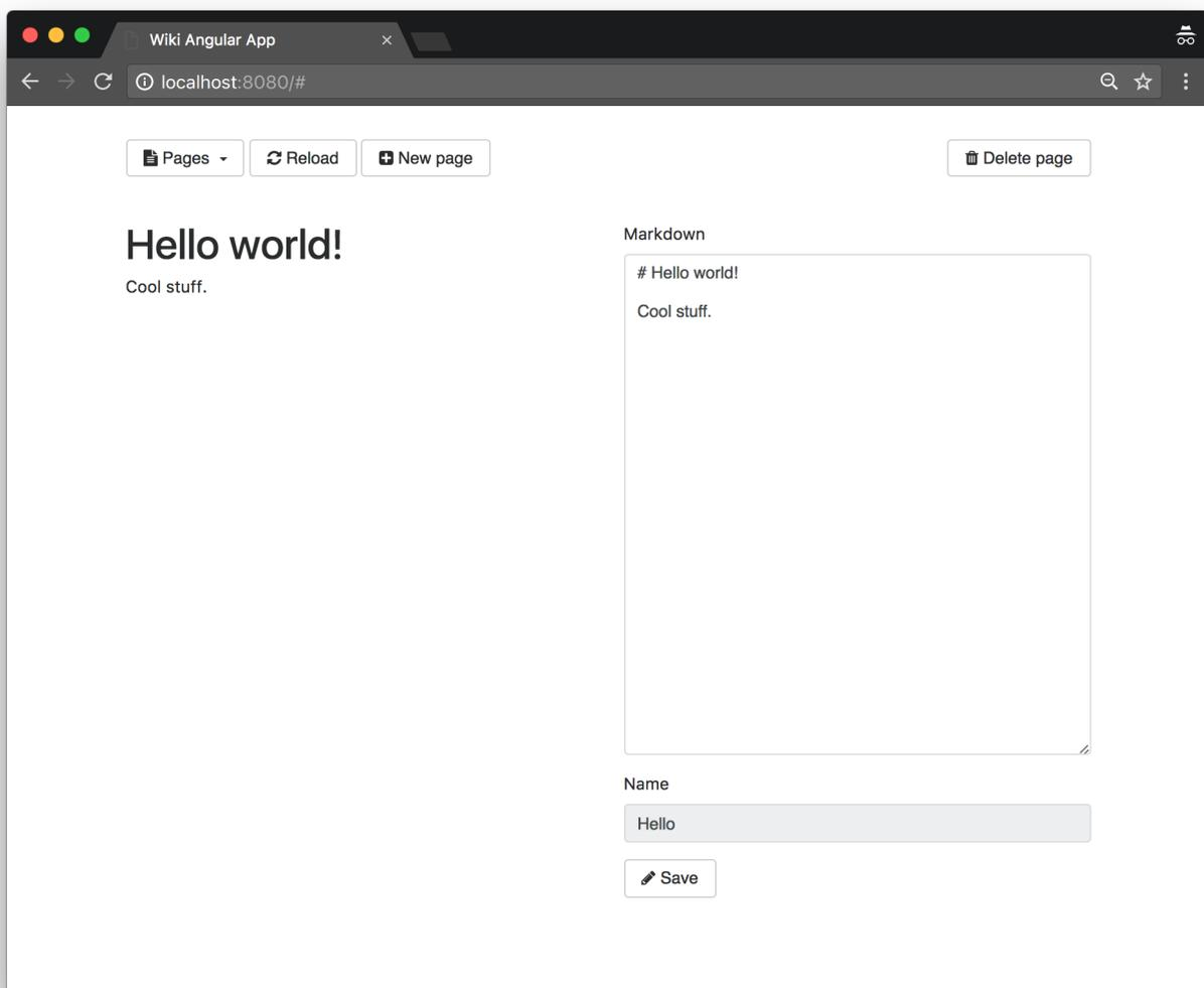
The HTML preview is being rendered by calling a new endpoint in our backend. Rendering is triggered when the Markdown editor text changes. To avoid overloading the backend with unnecessary requests when the user is busy typing Markdown, a delay is being introduced so as to only trigger the rendering when no change has been made during that delay.
